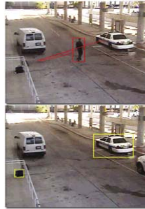
Multiple analytics modules applied to single camera. Shown: movement-in-zone, stopped vehicle and suspicious object
