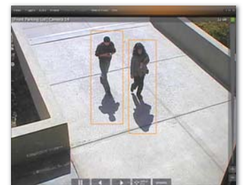
Content Analytics metadata displayed in Ocularis Client, with optical & digital PTZ controls
