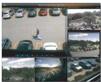
Ocularis Client: Instant Investigation Playback, virtual joystick-assisted optical PTZ and digital PTZ controls
